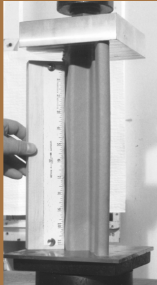
Figure 1.12—A study of corner posts was conducted by Urbanik et al. (2006) to understand the design principles of these packaging forms used to reinforce the strength of corrugated containers.
