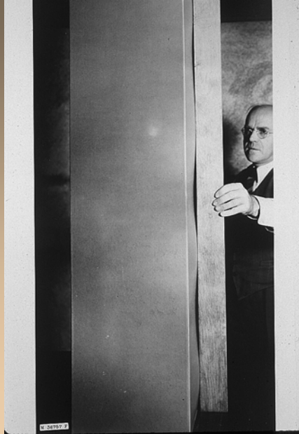
Figure 3.3—Buckling pattern with multiple waves developing along the side of a corrugated container subjected to top-to-bottom compression.
