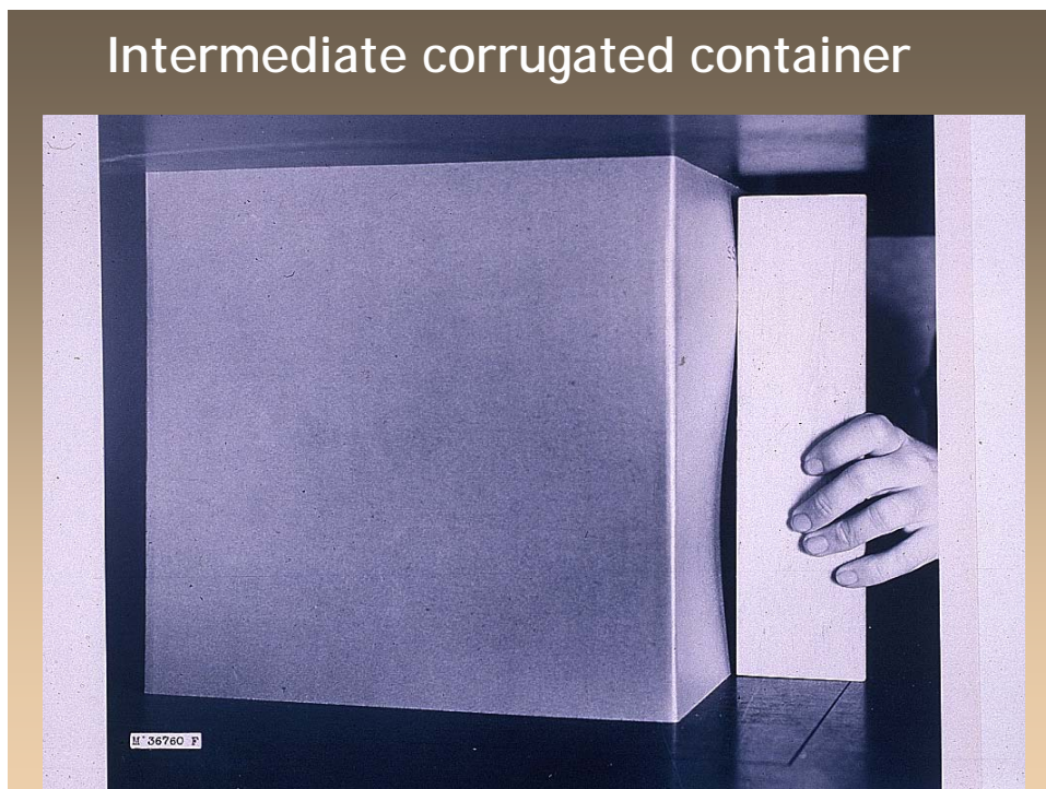
Figure 3.2—Buckling pattern with one wave developing along the side of a corrugated container subjected to top-to-bottom compression.
