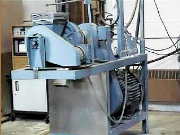
Figure 1.11—In a study by Urbanik and Won (2006), the FPL's experimental refiner was used to obtain a basic understanding of how the cost of refining energy compares to the cost of fiber in increasing paperboard strength.
